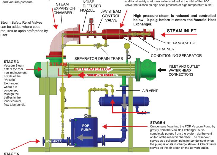
All condensate from the higher pressure traps is piped to the JCM Condensate Mixer where it is condensed below flash before discharge eliminating thermal hammer.
