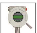
The multivariable flowmeters utilize three primary sensing elements—a vortex shedding velocity sensor, an RTD temperature sensor, and a solid-state pressure transducer—to measure the mass flow rate of gases, liquids and steam.
