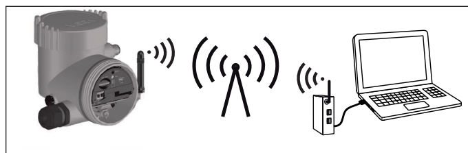
Fig. 33: Transmission of measured values and remote parameter adjustment of the sensor via mobile phone network.
