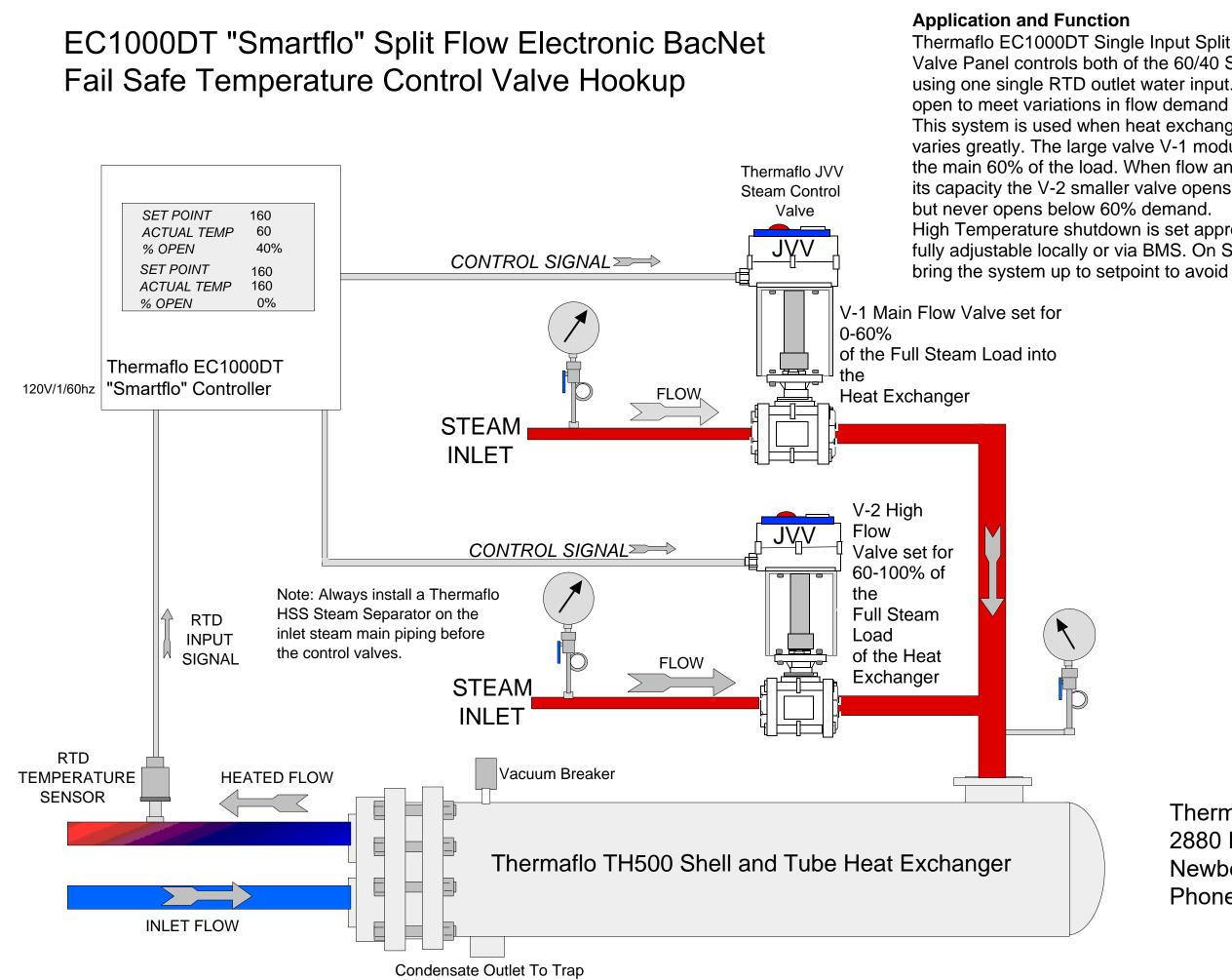
Thermaflo EC1000DT Single Input Split Range Electronic Steam Control Valve Panel controls both of the 60/40 Split Flow Valves independenly using one single RTD outlet water input. Valves can be set precisely to
