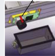
SUNTRAC Computer & Stepper Motor Drive (changes collector angles as it tracks the sun)
